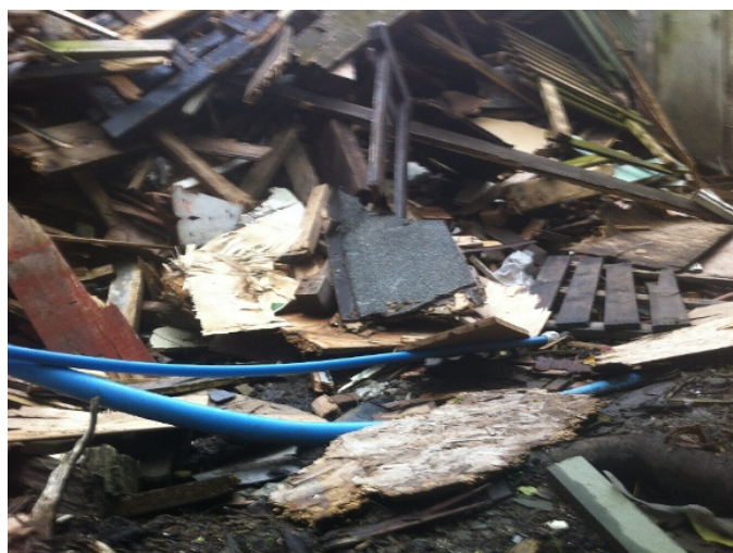
Photograph 5: Waste wood at Plevin chipping plant, Mossley. Dust emissions from this contain heavy metals, glass shards, paint flakes, textile fibres. MEAG
